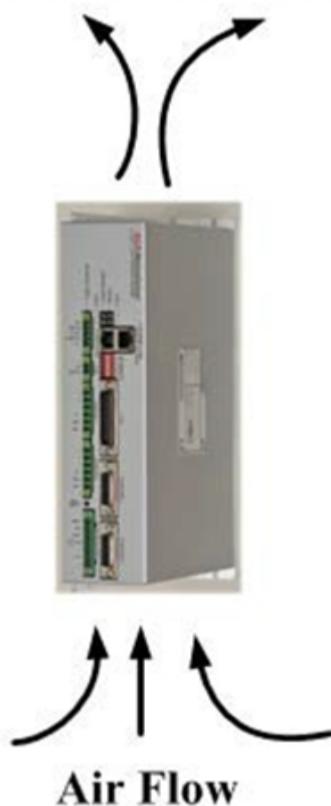
Figure 1-13. Vertical installation with cooling fan
